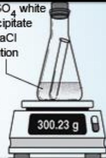
CaSO<sub>4</sub> white precipitate in NaCl solution
